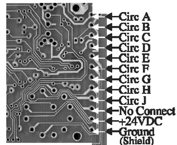
10. Multi-circuit products for flush mounting are equipped with 12-position plug-in terminal strips and are wired as shown above, right
