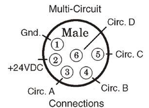
8. Multi-circuit enclosed products are equipped with Neutrik 6-pin XLR-type connectors wired as shown above, right.
