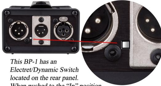
This BP-1 has an Electret/Dynamic Switch located on the rear panel. When pushed to the “In” position the unit will operate with an Electret Mic. When in the “Out” position the unit will operate with a standard dynamic Mic.
