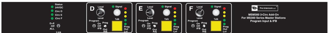
The MSM301 needs to be located close to the MS301 and connects to it via a single multi-pin cable, which is provided.
